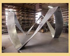
A high-end department store requested a unique table with a base that is a perfect circle when one looks straight down through a tempered glass top. The base is a five-foot continuous circle with no visible seams, stands two feet tall, and is crafted out of <sup>1</sup>/<sub>4</sub>" x 6" steel. The steel was brass-plated and chemically oxidized black.
