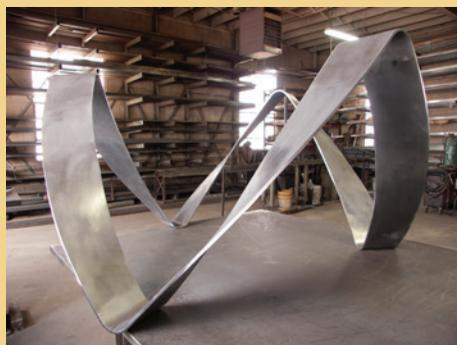
A high-end department store requested a unique table with a base that is a perfect circle when one looks straight down through a tempered glass top. The base is a five-foot continuous circle with no visible seams, stands two feet tall, and is crafted out of 1/4" x 6" steel. The steel was brass-plated and chemically oxidized black.
