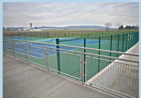
**TECHNICAL DETAILS:** All railings were core drilled with diamond core bits and poured into concrete with Super Por-Rok®, a self-sealing, anchoring cement.
