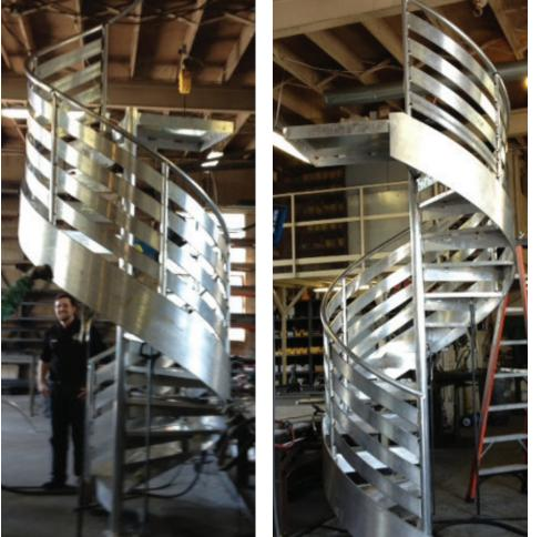
The entire staircase was powder coated and then the stringer, posts, and steps were painted to achieve a two-toned look. Shrock provided the support for the treads that are finished out in wood to match the flooring for an elegant look.
